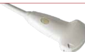
CA631 (1-8 MHz) Abdominal, Ob/Gyn, Vascular, Contrast Agents Procedures Variable-Band Convex Array
